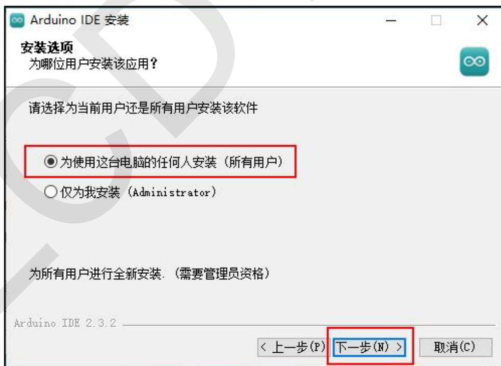
Picture2.3 Arduino IDE Software installation user selection
