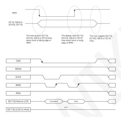
The timing of the parallel port communication read mode is shown in the figure below:
