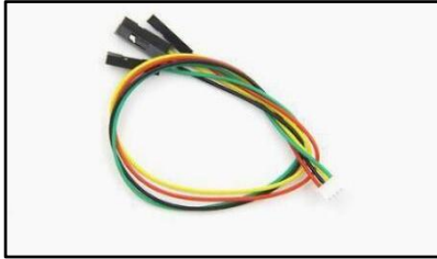
Figure 1.2 4P 1.25mm to 2.54mm Terminal Wire
