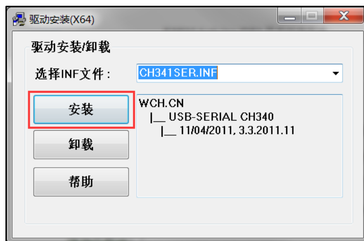
Figure 2 Installing the CH340C driver
