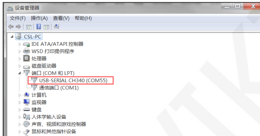
Figure 3 Identifying CH340 ports
