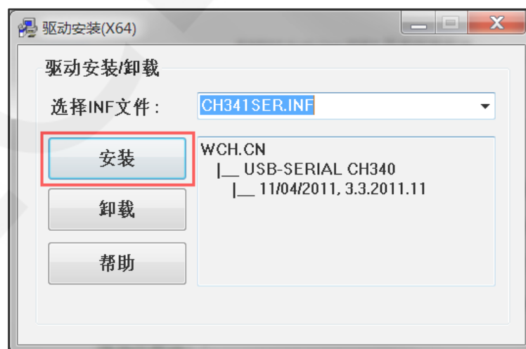
Figure 2 Installing the CH340C driver
