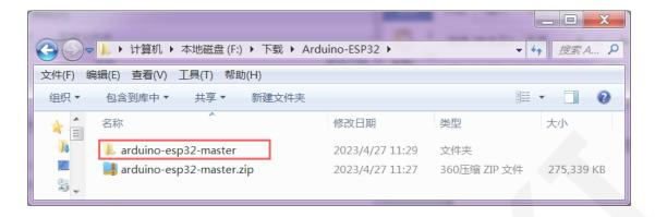
C. Open the Arduino IED installation directory, create a new espressif directory in the hardware directory, and then create an esp32 directory in the espressif directory. Finally, copy all the support library files extracted in the previous step (i.e. all files in the arduino-esp32-master directory) to the esp32 directory, as shown in the following figure:
