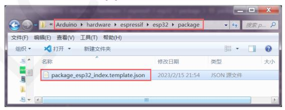
B. Open "package\_esp32\_index.template.json" file, Find the download links for the three files: "xtensa-esp32-elf-gcc "," esptool\_py ", and" mkspiffs". Wherein: xtensa-esp32-elf-gcc is the ESP32 cross compilation toolchain esptool\_py is a tool for burning (downloading) ESP32 software mkspiffs is the file system used on SPI NOR flash devices
