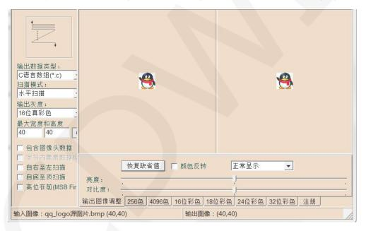
The Image2Lcd software needs to be set to scan horizontally, from left to right, from top to bottom, and with low bits in front.
