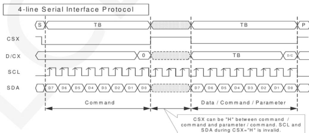
CSX is a slave chip selection, and the chip will only be enabled when CSX is at low
