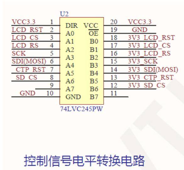
U2 is a level conversion IC that converts between 5V and 3.3V. This circuit only uses the one-way function of 5V to 3.3V, and the signals that the module needs to write are converted through this circuit.
