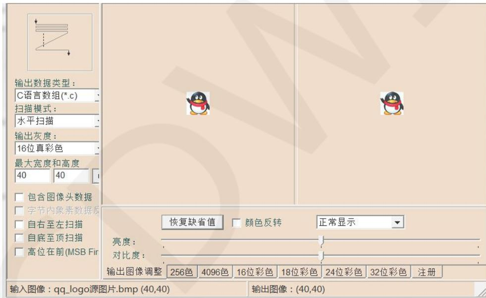
The Image2Lcd software needs to be set to scan horizontally, from left to right, from top to bottom, and with low bits in front.
