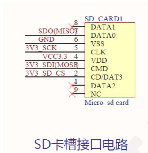
SD\_CARD1 is a Micro SD card slot for inserting Micro SD cards, making it easy to use SD card expansion functions. The SPI bus and LCD used are shared.
