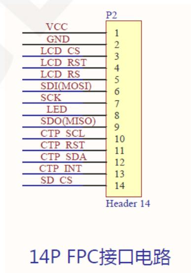
P2 is the module 14P FPC cable interface, which can only be connected to the main control through the FPC cable.
