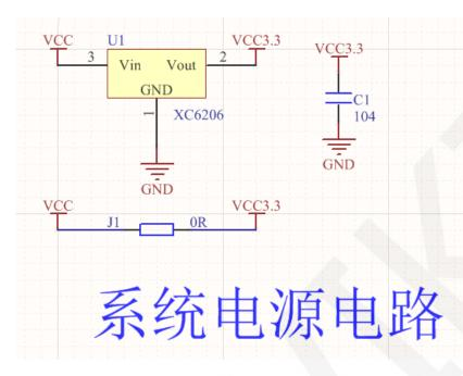
This circuit is a module system power regulator circuit, with U1 as the regulator, which can convert external input 5V or 3.3V voltage into 3.3V output, and C1 as the bypass filter capacitor.
