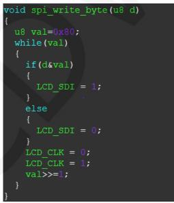
If the transmitted data bit is 1, the SPI data pin is pulled high. When it is 0, the SPI data pin is pulled low, one byte of data is transferred each time, the upper bit is first, and one bit of data is transmitted on each rising edge of the clock.
