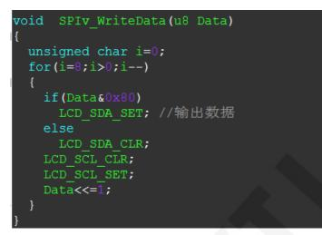
If the transmitted data bit is 1, the SPI data pin is pulled high. When it is 0, the SPI data pin is pulled low, one byte of data is transferred each time, the upper bit is first, and one bit of data is transmitted on each rising edge of the clock.
