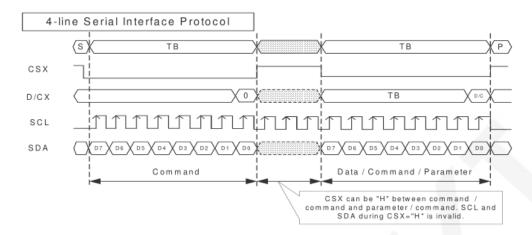
CSX is a slave chip select, and the chip is enabled only when CSX is low.
