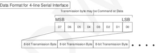
The high position is in front and transmitted first.
