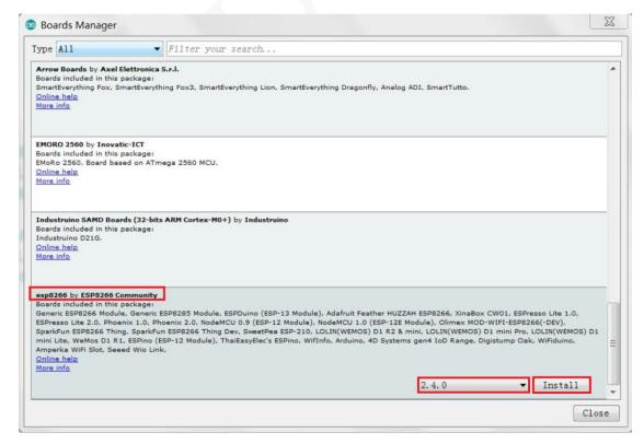
F. After successful installation, the corresponding development board model can be found in IDE, As shown in the following figure:
