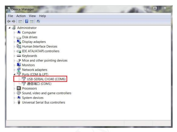
B. Open Arduino IDE, click Tools, Set as shown below (As long as the driver is installed successfully, the Port will be automatically recognized, Select a com that is consistent with the device manager display, The larger the Upload Speed, the faster the download)
