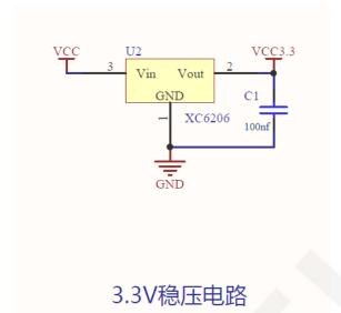
This circuit is used to stabilize the input voltage of the module, where VCC is the external input voltage, VCC3.3V is the module input voltage, and C1 is the bypass filter capacitor. VCC can be connected to 5V or 3.3V, and it is recommended to connect to 5V because only by connecting to 5V can VCC3.3 output 3.3V. If connected to 3.3V, VCC3.3 output voltage will be less than 3.3V, which will cause the backlight brightness of the LCD screen to darken.
