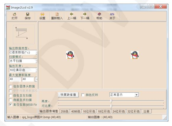
The Image2Lcd software needs to be set to scan horizontally, from left to right, from top to bottom, and with high bits in front.
