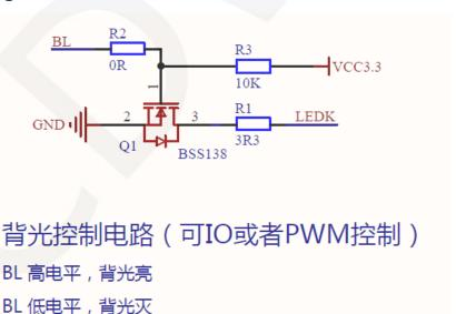
R2 is reserved for compatibility with J3Y control circuits, directly using a 0 ohm resistor. R1 is the backlight current limiting resistor, R3 is the pull-up resistor,
