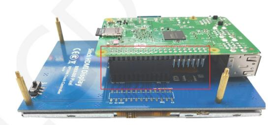
2) Connect The LCD and Raspberry Pi with the HDMI adapter.
