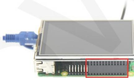
Insert the MicroSD card that burns the official system image file, connect the network cable, and connect the power supply.
