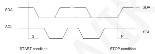
When both the data line and clock line of the IIC remain at high level, the IIC is in an idle state. At this time, the data line changes from high level to low level, and the clock line continues to remain at high level. The IIC bus starts data transmission. At that time, the clock line remained at high level, the data line changed from low level to high level, and the IIC bus stopped data transmission.
