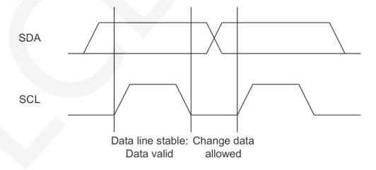
Send 1 bit of data for each clock pulse (the process of pulling up and down). At that time, the clock line was at high power level, and the data line must remain stable.
