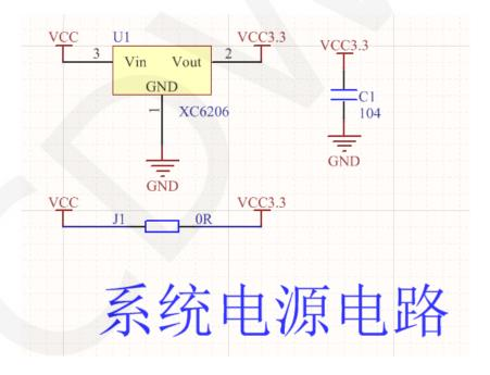
This circuit is a module system power regulator circuit, with U1 as the regulator, which can convert external input 5V or 3.3V voltage into 3.3V output, and C1 as the bypass filter capacitor.
