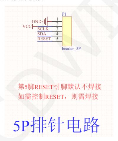
This is a 5P 2.54mm spacing row pin interface circuit used to connect to the main control. Among them, P1 is a 5P pin, and 1-5 pins are GND, VCC, SCL, SDA, and RESET respectively. Due to the internal reset circuit of the module, the RESET pin is not soldered by default. If you want to control the RESET function in the program, you need to solder the pin and connect it to the GPIO port.
